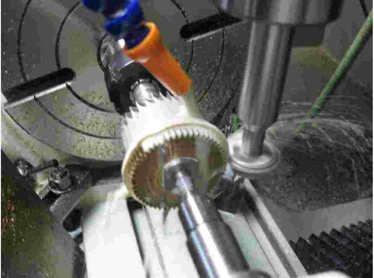
Photo 8 Cutting the new barrel wheel.
