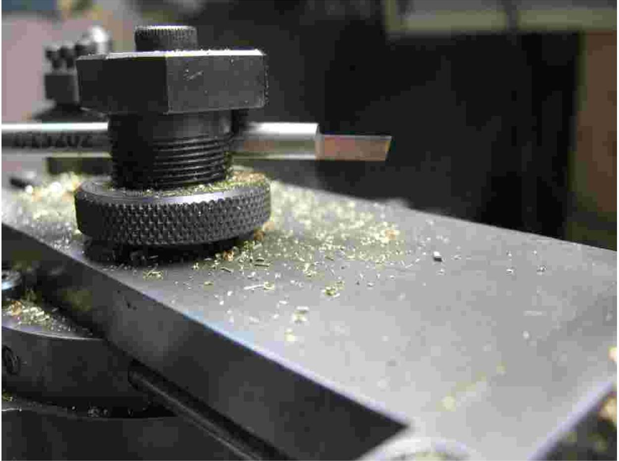
Photo 1 3/16" Drill rod cut off tool, .0135" thick
