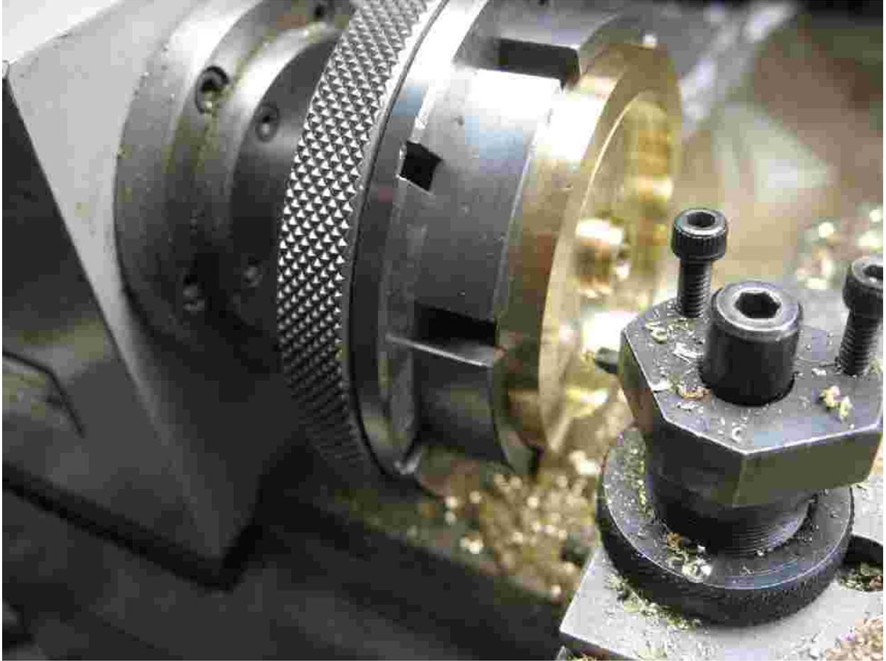
Photo 7 Machining the new wheel blank and machining the recess
