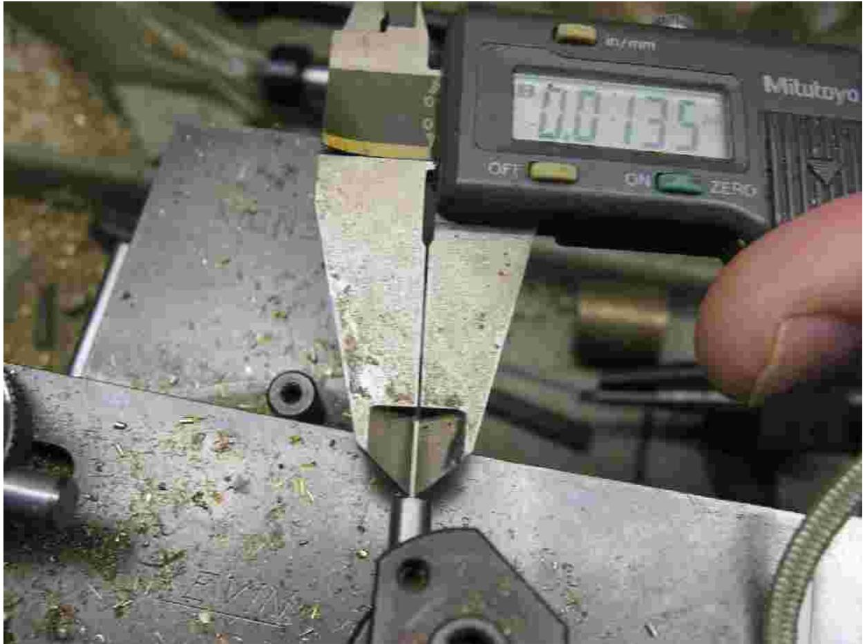
Photo 2 Top view showing the thin sharp blade of the cut off tool
