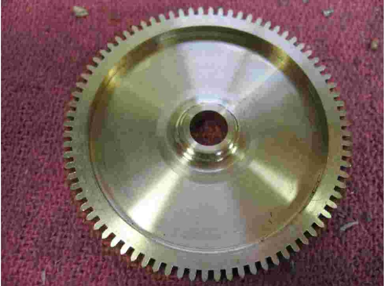
Photo 10 Wheel is ready to have a final step machined to match the OD of the step machined on the barrel itself. The step is then soft soldered to the barrel.
