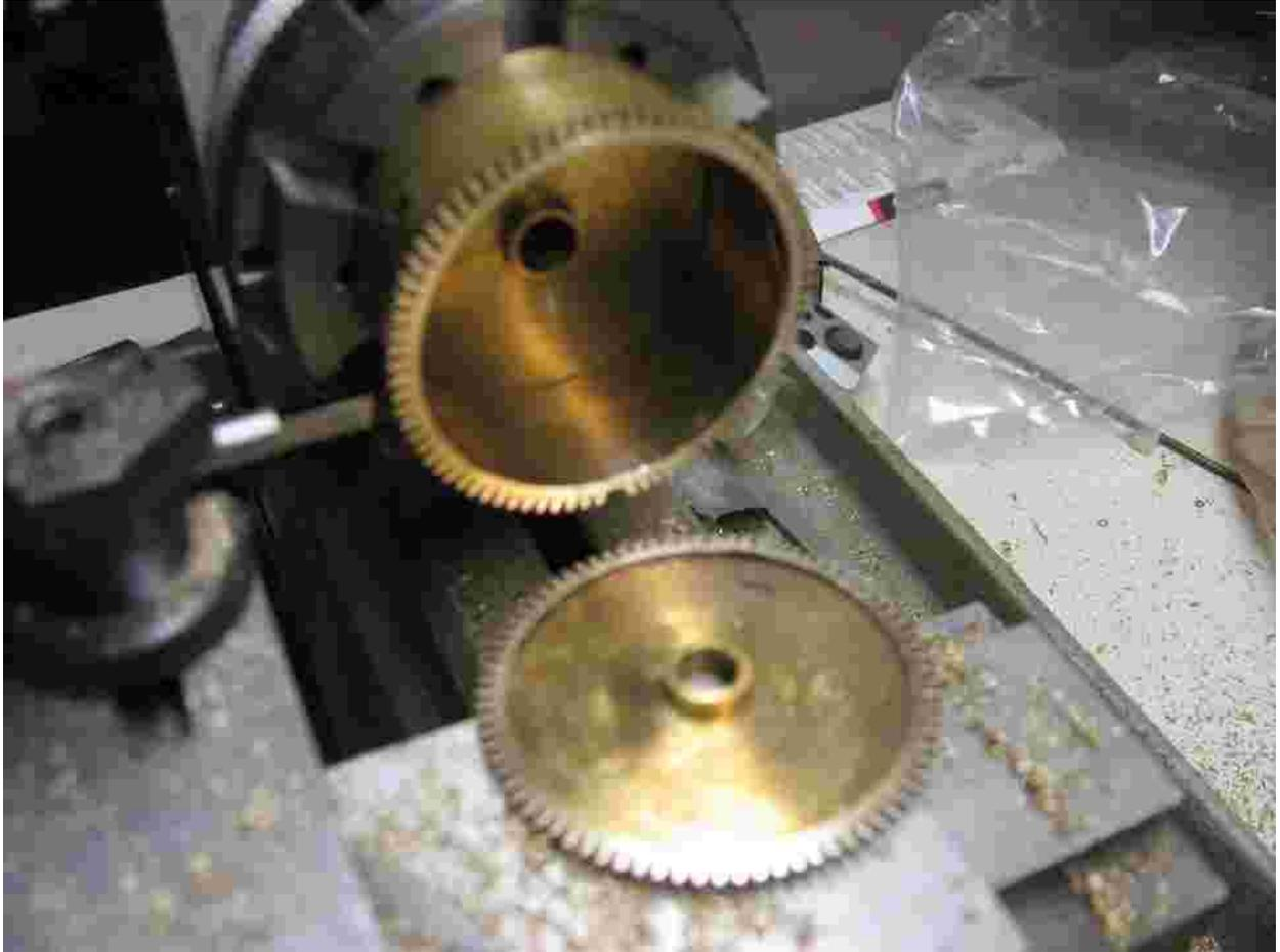
Photo 3 Removing the damaged wheel / barrel face
