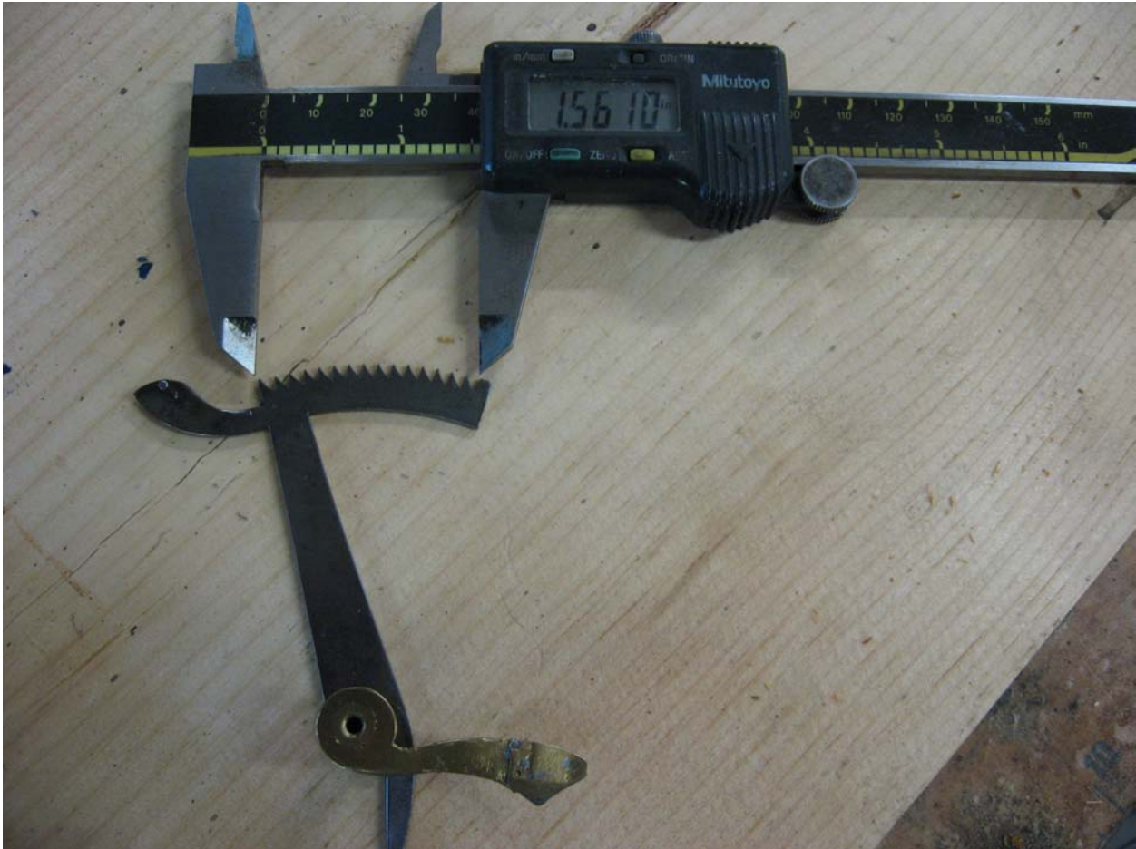
Measure the span of the teeth, count the teeth
